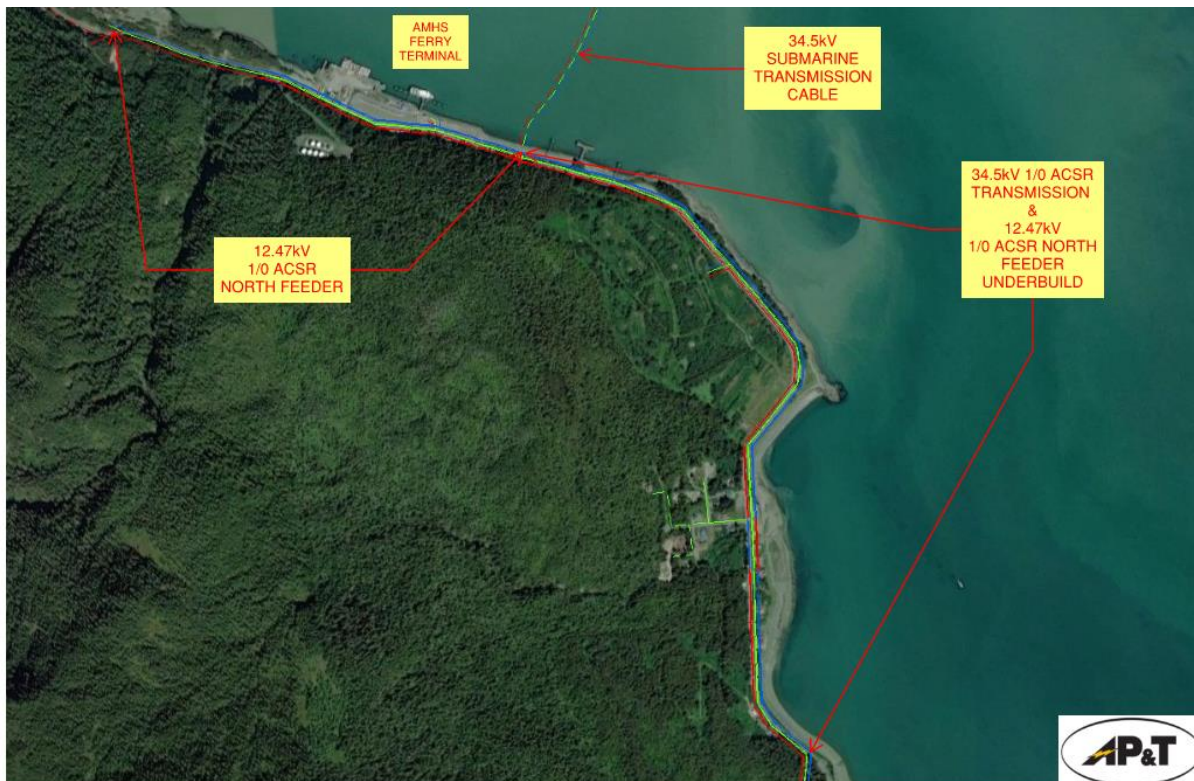
Figure 3: AP&T Infrastructure near the AMHS Terminal in Haines (Provided by AP&T)
